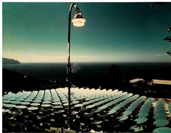
Fig. 8. The third iteration of Francia's Genoa PT test facility using a receiver of the type later installed at Georgia Tech in the USA.
