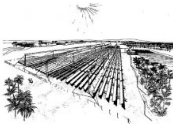
Fig. 21. Artist's rendering of an Linear Fresnel Concentrator solar power plant designed by Giovanni Francia and collaborators (Circa 1965). Source: The Francia Archives donated by his heirs.
